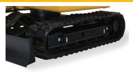
Depending on the customers application, the Cat 308E2 CR has three different track options to choose from, allowing the correct machine configuration to suit the job.
